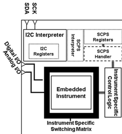
The proposed IP interprets I2C transactions as a means for instrument specific control logic management, through the update of a structured set of registers/pointers; permitting the sequencing of inter/intra-modular task sets.
